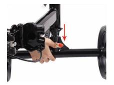
Figure 3. Secure the steering column by pushing the clamp lever to the left which will allow the safety pin to lock into place. Raise the clamp lever upward into the "U" shaped slot and tighten by turning clockwise. Push the clamp lever down firmly to secure the steering column.
