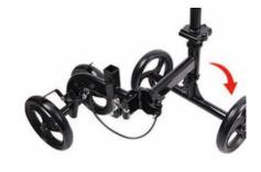
Figure 5. Squeeze the hinge pin down which will lock it into place. Tighten the lever until it is securely locked into place.
