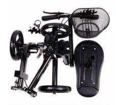
Figure 2. Pull down on the guide pin ring and turn the front axle so that the guide pin ring is between the guide stops. Release the guide pin ring and your front axle is set in the proper position.
