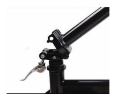
Figure 4. Secure the center frame hinge by connecting the front and rear frame sections by closing the center frame hinge.
