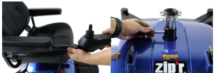
Figure 2. To insert your batteries, remove the joystick controller from the armrest. Afterwards remove the vinyl seat and chrome seat post from the base of the Zipr PC.
