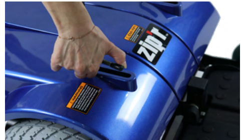
Figure 3. Adjust both freewheel levers, one located on each side so that both levers are pointing forward, so that the motor is disengaged.
