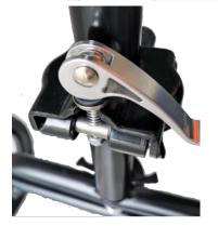
Figure 5. Insert the handlebar into the steering column. Adjust the handlebar to a comfortable height, then secure it into place by attaching and tightening the locking knob ensuring that it goes all the way through the pinhole.
