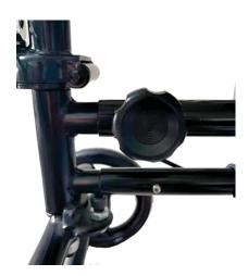
Figure 2. Install the brake cable clip to the lower mainframe.
