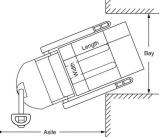
Aisle dimensions listed above assume the minimum bay width to be straddle OD plus 127mm (64mm on each either side of straddle leg). Straddle OD is the load width plus 203mm. Truck perform ance may vary due to application require ments' and changes in model design.
