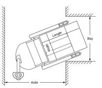
Aisle dimensions listed above assume the minimum bay width to be straddle OD plus 127mm(64mm on each either side of straddle leg). Straddle OD is the load width plus 2 0 3 mm. Truck performance may vary due to application requirements' and changes in model design.
