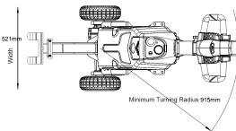
Stability Caster Track Width 216mm Drive Tire Track Width 429mm
