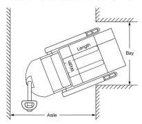
Aisle dimensions listed above assume the minimum bay width to be straddle OD plus 127mm (64mm on each either side of straddle leg). Truck performance may vary due to application requirements' and changes in model design.
