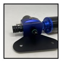
21. Now install the regulator bracket in the car using the two bolts found near the transmission as seen in these photos. The bolts used are M8x1.25x16mm Stainless Steel Flange Nuts. You may also install the primary feed line and return line as seen in the photos at this time.
