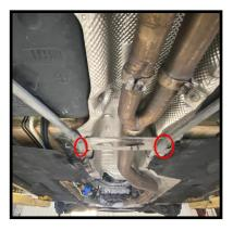
16. Loosen the rear nuts (do not remove), and loosen the front tank brackets. This will allow the tank to sag down towards the front of the tank.
