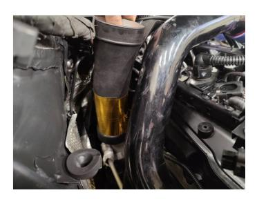
22. Remove the bolt holding the front charge tube on the passenger side of the engine to the engine block using a T27 Torx. It is the charge tube leading to the intercooler. (Torque Spec: 10Nm)
