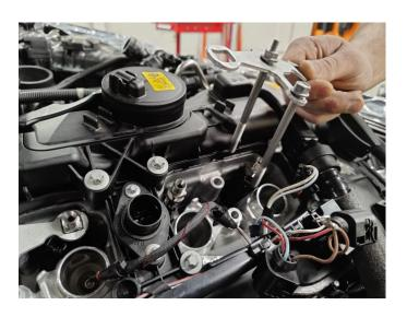
39. Grab the threads on the top of the injector and pull it out of its seated position. (If you are unable to pull the injector out by hand, you may use an injector removal tool—please follow instructions associated with that tool)
