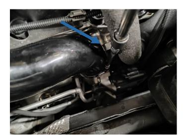
23. Use an Allen 5 to remove the back charge tube on passenger side at the engine (Torque Spec: 10 Nm)
