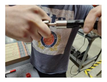
43. Install each injector within 20 seconds of pulling the compression toll off the stem of the injector. Place your new injector with the connector facing to the left of the coil pack socket. There is space for the solenoid connector in its seating location. This will make it easier to seat correctly.
