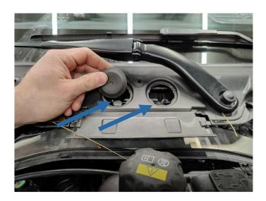
11. Remove wiper cowl bracket bolts using a 16mm socket.
