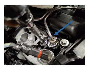
35. Remove the bolts holding the rail in place using a 11mm socket. (Torque Spec: 13 Nm)
