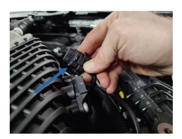
18. Remove the coolant lines at the front of the intercooler. Use a pick tool to pull the latch out of the fitting to free it from the intercooler.
