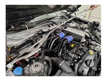
13. Remove the bolts holding the lower section of the wiper cowl using a 10mm socket. Remove it from the engine bay.
