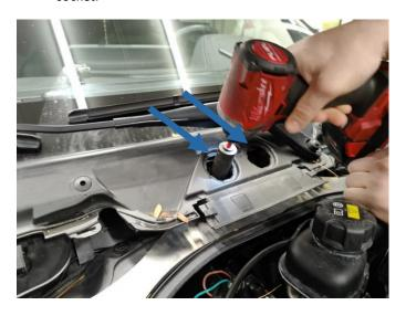
12. Remove the strut bracket from the engine bay
