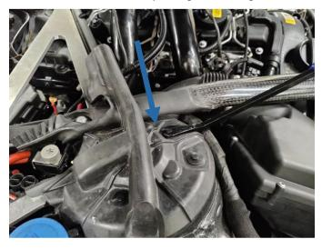
6. Remove retaining clips to remove the fender edge trim
