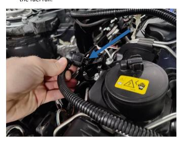
26. Disconnect pressure sensor on the back of the fuel rail.
