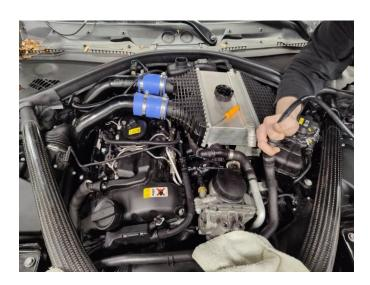
15. Remove the hose clamp bolts using an 8mm socket to disconnect the charge tubes from the intercooler.
