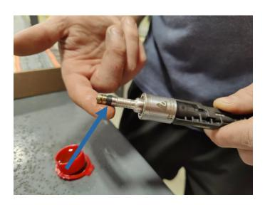
42. Place the compression toll over the stem, twisting clockwise as you press. Stop with injector fully inserted for 15 seconds. Afterwards remove the injector while twisting clockwise.
