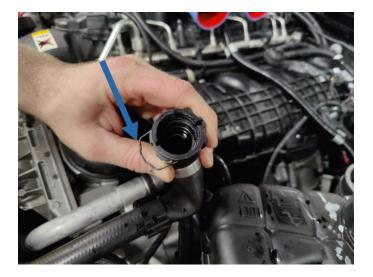
19. Remove the hose clamp connecting the charge tube to the airbox using a 6mm socket.
