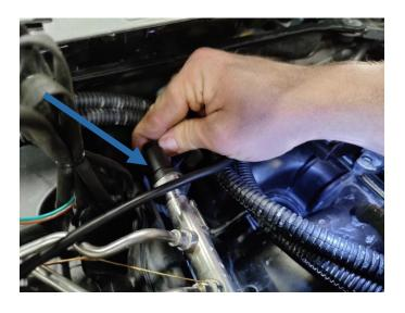
27. Loosen the compression nuts for both high-pressure fuel lines that feed into the fuel rail using a 18mm wrench. Use a rag or absorbent towel to catch any fuel that may exit the lines. (Torque Spec: 30 Nm)
