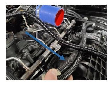
25. Once the wires are free, remove the connector for the variable vanos lift control valve and pull it away from the fuel rail.
