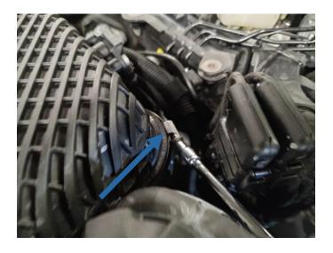
17. Remove the manifold absolute pressure sensor at the back of the intercooler.
