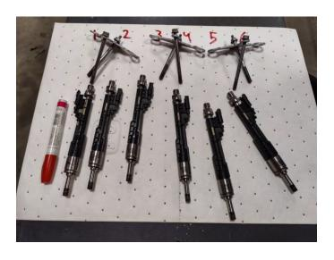
41. Place engine oil onto the stem of the injectors by using your finger to spread the oil across the stem.
