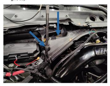
14. Drain coolant from the intercooler to prevent any coolant leaking once the intercooler is removed.
