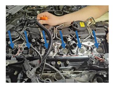
33. Use a pick tool to pull the tab on the injector solenoid connectors. As this is done pull the connectors out to disconnect them.
