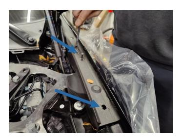
7. Remove cross bar by removing the 7 bolts securing into the engine bay using a 13mm socket. (Torque Spec: 28Nm
