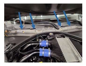
Remove retainment cable from the rubber insulator between the wiper cowl and the engine
