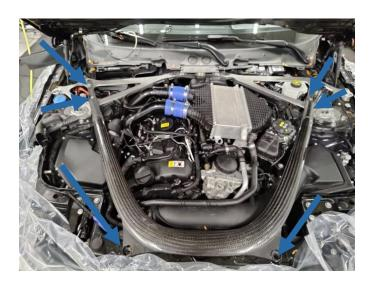
8. Remove Bolts from the driver and passenger side strut tower using a 13mm socket (Torque Spec: 56 Nm)
