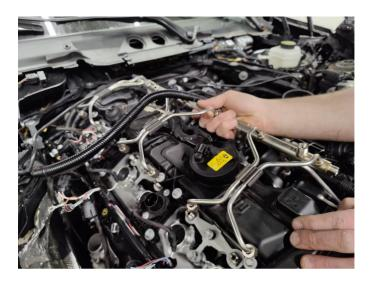
37. Remove the bolts holding the injector bracket over the injector using a 10mm socket. (Torque Spec: 13 Nm)
