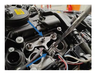
38. Pull the brackets off the injectors.
