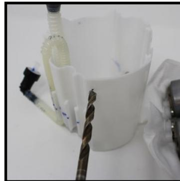
25. Re-install the pump assembly into the bucket, again ensuring proper rotation of the assembly inside the bucket. Line the drilled holes from the previous step with the holes in the bracket and insert the provided nylon rivets.
