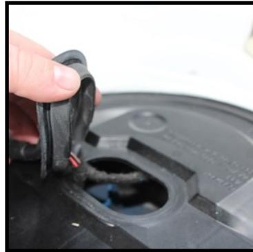
4. Remove the plastic cover by pushing the cover towards the rear of the car firmly and pulling up on the front. Be careful not to break the plastic tabs from the cover.
