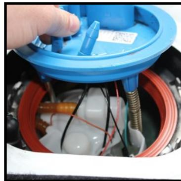
9. **DO NOT LIFT THE ASSEMBLY OUT OF THE TANK AT THIS TIME** as damage can be caused by the fuel float being caught on the inside of the tank! Disconnect the fuel float from the sending unit by using a small screwdriver or pick tool and popping it up from the lock, then remove the float from the tank first.
