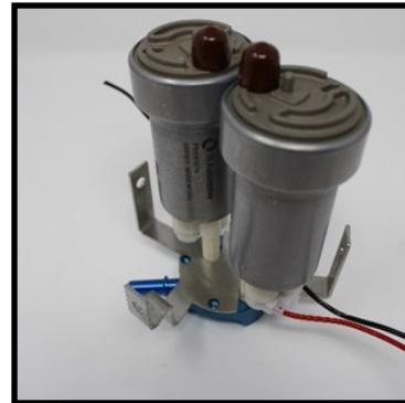
19. Install and tighten the 2 screws on the side of the manifold with the flat. Then start the first threads of a screw in either of the two other holes. Slip the pump support between the two pumps hooking it under the partial installed screw. With the pump support in place, line up the mount with the last screw hole and insert the screw and tighten the two screws securing the support. (**Note: The pumps can twist as needed to provide better access to the screws**)
