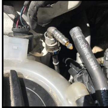
9. Grab firmly onto the metal fuel line, and pull. Some wiggling is required and a second set of hands to reach under the car and make sure the fitting starts down the frame rail can be useful. Pull until the fuel line is completely removed from the car and discard.
