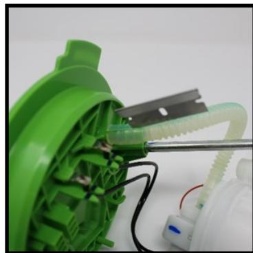
22. Install the supplied corrugated fuel line over the barbed port of the top hat where the factory line was removed. Secure the line with the provided crimp style hose clamp (note the direction the quick connect fitting faces in the below photo).
