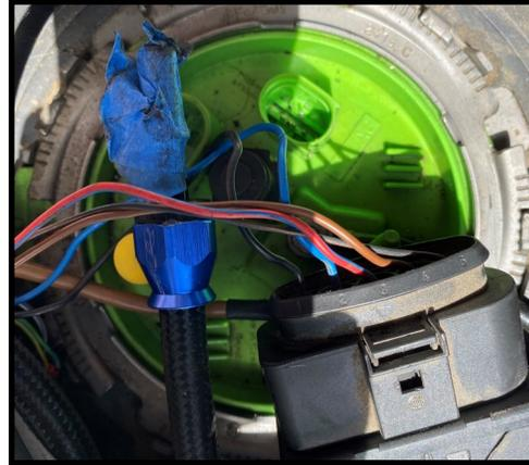
10. Use the 90 degree double quick connect to install the return line on the added return port. Run Feed Line 1 (short feed line) from the top of the tank down to the bottom of the tank. (Female Quick connect goes to fuel pump top hat). Connect 90 degree an fitting to input of fuel filter and output of filter to the female AN6 of Feed Line 2.
