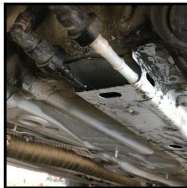
3. Locate and disconnect the quick connect fitting located slightly in front of the tank before the line enters the frame rail.
