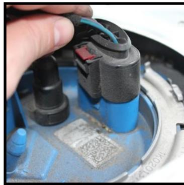
6. With the harness now disconnected from the fuel pump, start the car. This is to de-pressure the fuel line. It can take a few minutes for the car to stall out. Ignore any dash lights resulting from the plug to the pump being disconnected. While the car is idling, use this time to push the rubber grommet through the dust cover and take a rag to clean the top of the fuel pump assembly.
