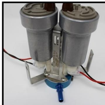
20. Secure the pumps with the provided nylon zip ties to prevent any possible lateral movement in the pump reducing strain on the pump neck. Then install the fuel socks on both pumps.
