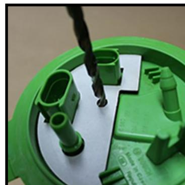
29. Drill 2 holes in the flat portion of the top hat for the provided stainless hardware used to provide power to the secondary pump. Ensure the drill bit selected is close in size to the actual bolts provided and that there will be no interference with connectors once assembled. Crimp the provided ring terminals onto the secondary pump and assemble as shown using a sharpie to mark on the outside of the top hat which side is positive and negative.
