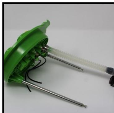
23. Insert the completed pump assembly into the bucket. Ensure the orientation fo the pump assembly matches the photo below. (If installed backwards, you will not be able to fit the assembly in the tank later.)
