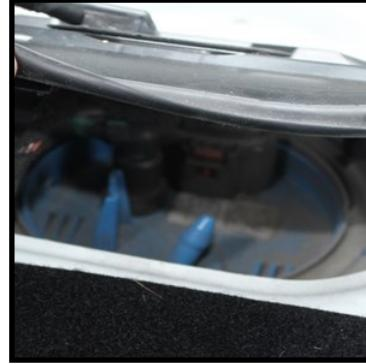
5. Using a flat blade screwdriver, pull up the red locking tab (it does not require much pressure). Then disconnect the electrical harness from the fuel pump
