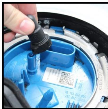
8. Using a large flat blade screw driver and hammer if needed tap the lock ring in a counter clockwise rotation until the ring is released. Remove the ring and the pump should be released (it will pull up easily as shown).
