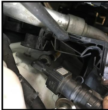
7. Pull up on the plastic fuel line shield to release this clip and continue to pull firmly until plastic fuel line shield has been removed from the car.
