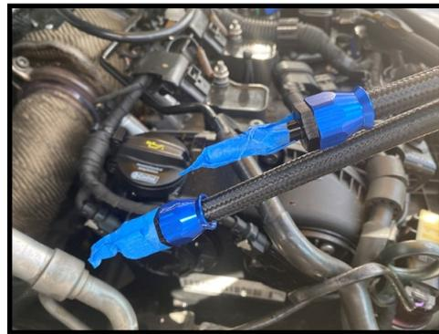
9. Tape the wire harness to one fuel line. (Set it back a couple of inches to prevent it from snagging. Then feed both lines down the frame rail until they come out the other end. \*\*Lines should be staggered so they are able to fit through frame rail. These will likely get stuck towards the end of the frame rail, and may require some pull back twist and try again motions. Also a second set of hands can be helpful for this.
