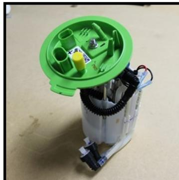
33. Install the pump back into the car using steps 1-10 above in reverse as a guide. Use caution not to damage the fuel float during install. The tab on the top hat of the pump should face the rear of the car when installed properly. If the location of the tab does not face the rear of the car, the fuel gauge will not read correctly and damage could occur.
