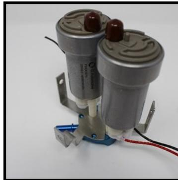
19. Install and tighten the 2 screws on the side of the manifold with the flat. Then start the first threads of a screw in either of the two other holes. Slip the pump support between the two pumps hook it under the partial installed screw. With the pump support in place, line up the mount with the last screw hole and insert the screw and tighten the two screws securing the support. **(Note: The pumps can twist as needed to provide better access to the screws)**
