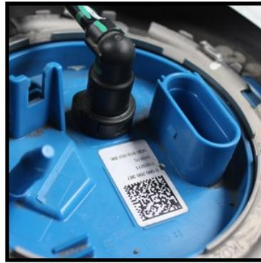
7. Once the car stalls out it is time to disconnect the fuel line. The line will still have a decent amount of pressure use a fresh rag to cover the assembly and soak up any fuel. Quick connects always work best by pushing down first on the connector then pushing in on the release and pulling up. Pull up slowly as full will spray out and have it covered with a rag to not make a mess. Allow the remaining fuel to soak into the rag so that it can be discarded.
