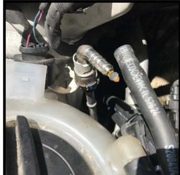
9. Grab firmly onto the metal fuel line, and pull. Some wiggling is required and a second set of hands to reach under the car and make sure the fitting starts down the frame rail can be useful. Pull until the fuel line is completely removed from the car and discard.
