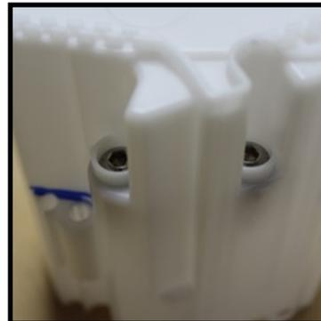
16. Install the corrugated tube with anodized venturi fitting as shown in the photo below and secure as seen with provided zip tie. Then reinstall venturi and lines as shown pushing firmly on the venturi until it snaps into place.
