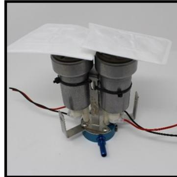
21. Cut the factory fuel pump wires cutting roughly 2" from the actual pump. Then using a razor cut a slit in the fuel tube as shown and remove the tube from the top hat.
