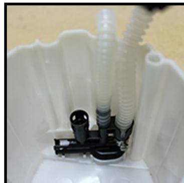
17. Install the two male quick connect fittings and 1/8" NPT plug as seen in the photo below. Use Teflon tape to seal the NPT plug. The quick connect fittings should not need any tools to tighten, however if needed, protect the fitting with a leather work glove and grip with pliers to tighten (do not use a towel or damage may occur!)
