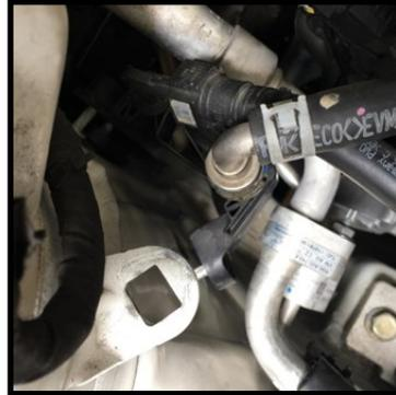
6. Release the fuel line and emissions line from the inside of the plastic fuel line shield.
