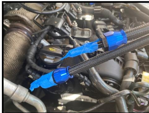
9. Tape the wire harness to one fuel line. (Set it back a couple of inches to prevent it from snagging. Then feed both lines down the frame rail until they come out the other end. \*\*Lines should be staggered so they are able to fit through frame rail. These will likely get stuck towards the end of the frame rail, and may require some pull back twist and try again motions. Also a second set of hands can be helpful for this.
