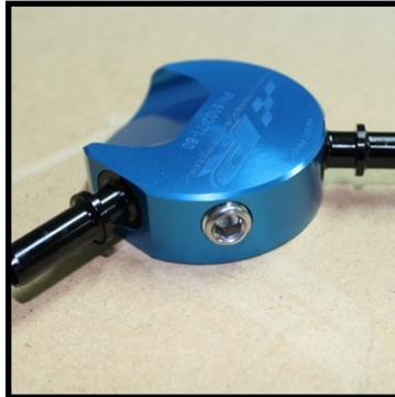
18. Install one pump into the manifold pushing until the lip of the pump is flush with the surface of the manifold. With the pump fully inserted line up the flat of the mounting bracket with the flat edge of the manifold and slip around the neck of the pump. While tilting the bracket insert the next pump and insert the second pump fully.
