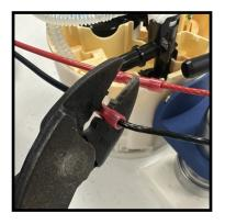
25. Using a zip tie, secure the wiring from the secondary pump to the factory wiring near the center of the factory wiring. This step is not required but provides clean install while reducing possibility of wiring getting in the way of the fuel float.
