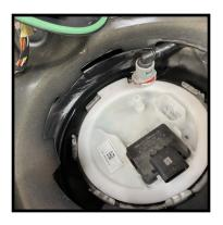
7. If you purchased a lock ring removal tool this step is a breeze, simply align the tool with the tabs on the outside of the lock ring and turn counter clockwise (using a large ratchet) to remove the lock ring. If you do not have a lock ring tool, we recommend using a socket wrench extension placing the female end against the edge of the tab and hitting with a hammer until unlocked. Once unlocked remove the lockring and set to the side.
