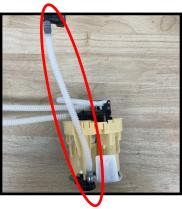
15. The second fuel line will be installed onto the middle barb where the line was previously removed. The opening of the quick connect fitting will face the front of the assembly. (Opposite the float side) Again, heating the line slightly will ease installation. Once proper orientation is achieved, secure in place with the pinch clamp
