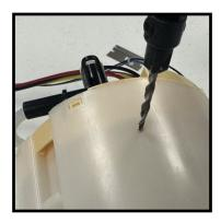
19. Drill the hole marked in step 9, for metal rivets you can start and finish with 1/8" drill bit. For plastic rivets you will start with 1/8" working up in size until you reach the final size of 1/4".
