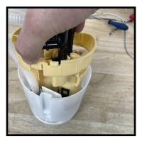
13. Using a razor blade remove the middle line on the barbed ports that connect to the lower venturi. Do this to both sides of this line, removing the line completely.
