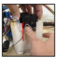
12. Remove the internal components from the bucket by releasing the 4 tabs around the lip of the bucket. This can be achieved by using a small flat head screwdriver or pick and wedging them at the two locking points closes to the float. Using another screwdriver gently pry the two tabs at the front of the bucket until all have been unseated and pull up on the components. (It will all come out together)
