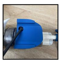
24. Place the fuel pump on the sheet metal hanger (note it will not sit all the way down at the bottom of the hanger). Then attach the pump wires to the bulkhead wires using the supplied butt connectors or spades by crimping the connectors to the wires.
