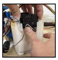
12. Remove the internal components from the bucket by releasing the 4 tabs around the lip of the bucket. This can be achieved by using a small flat head screwdriver or pick and wedging them at the two locking points closes to the float. Using another screwdriver gently pry the two tabs at the front of the bucket until all have been unseated and pull up on the components. (It will all come out together)
