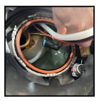
9. The left side of the car has a fuel level sensor which has wires the run to the drivers side of the car and attach to the fuel pump top hat. Follow these wires and disconnect the connector associated with them by sticking a small flat head screwdriver in the notch on the top side near the latch and prying up carefully to release the connector from the top had. With the connector released pull the connector off the top hat.
