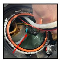
27. With the pumps back in the tank ensure there are no wires or hoses that can interfere with the fuel float. Reattach the fuel float connectors to the underside of the top hat. With both connectors reconnected and everything clear of the fuel float movement place the top hat back on the fuel tank with the tab pointing to the rear of the vehicle. Then reinstall the fuel pump locking ring ensuring it reaches the locking indention to ensure it seals properly to the fuel tank.
