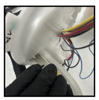
12. Once the line is removed, cut the barbed fitting on the top hat off using a rotary tool or other tool that can make clean cut. Note: Do not cut into the underside of the top hat as the surface will need to be able to seal against o-ring later.
