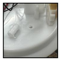
13. With the barbed fitting cut off, start with a drill bit slightly larger than the hole drilling through the top hat. Keep stepping up one bit size at a time until you reach 1/2" for the final size. Be careful of the wires while drilling so they do not get damaged Note: Using a large bit and not working up in size will crack plastic
