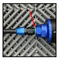
34. With both lines attached to the fuel filter, located the supplied fuel filter bracket. Install the bracket on the 2 studs coming down from the bottom of the car using the supplied nuts. The filter body has a groove which will interlock with the filter bracket when aligned properly. Nuts should be tightened snugly but do not require excessive torque.
