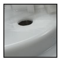
15. Make a mark in the center of the area shown below (center of slightly raised area). Start with a small drill bit and work up one size at a time until you reach the final size of 11/16". Using a razor or other tool deburr the drilled hole as needed. Note: Be careful not to catch wires under the tophat with drill bit (holding them out of the way is recommended).
