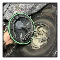
Disconnect the electrical wiring from the fuel pump by pulling up on the red locking tab, and then press on the release for the electrical connector while pushing down. While still pressing the release pull up to remove the connector from the pump.
