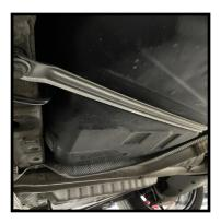
31. With all panels removed and the tank lowered, disconnect the stock plastic fuel line from the metal line located near the front left vehicle lift point. With the line disconnected start removing the line from each clip working towards the back. Continue removing the line from the clips in front of the fuel tank by moving the fuel tank for access ass needed.
