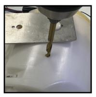
21. With the second hole drilled secure the sheet metal bracket to the outside of the bucket using either the metal rivets or the plastic rivets provided in the kit.
