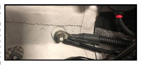
grounds on that stud appropriately and now place the nut back on and tighten to spec.
