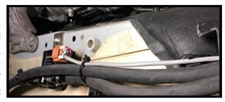
the firewall to the driver side of the engine bay. For those of you who mounted the ethanol sensor in the engine bay go ahead and make the connection. For the people who mounted it under the car, run the conduit down the tunnel with the feed line and connect it to the sensor.
