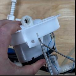
6. Disconnect venturi jet from venturi body by using a flathead screwdriver to press the clip in. Then remove the venturi jet from the venturi body. Remove the venturi body and components attached to the venturi body from the hose bundle.
