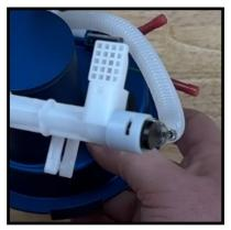
9. Using wire strippers, strip back a little bit of wire, and then crimp wire into a red barrel connector. There is no wire required to be connected to another wire, so long as both wires from the float are attached to both wires on the assembly you are good.
