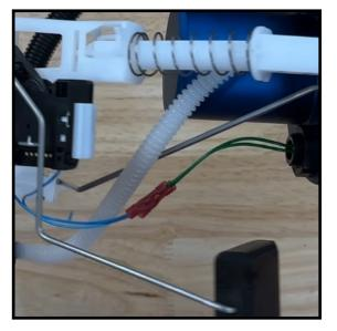
10. Attach the two fuel lines to bottom ports of assembly using a straight fitting from each hose. Route both lines and bundle together using zip ties attaching them to the stock venturi output line. It will look similar to how the factory assembly was before removing the venturi output line from the bundle.
