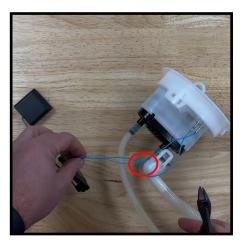
4. Using a small screwdriver to release the retaining clip and pull the arm down to remove the float arm from the assembly.
