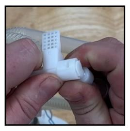
7. Moving to the new E9x / E8x Fuel Filter & Regulator, the first step is to install the float arm into the body. Depending on when your car was made, you may have to trim the corners of the float arm to fit with a razor blade. There should be little to no force to install, and it should click once seated.
