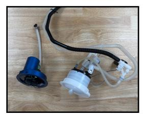
3. Cut the wires connected to the fuel float sensor. The wires should be cut to be equal length and as long as possible.
