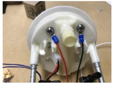
5. Install Y-Hose through the large hole between the pumps and the back of the bracket. (the straight goes to the stage 2 pump, and the y goes to the stage 3 pump) make sure it is ran to not interfere with the float assembly.
