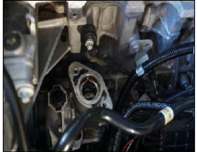
Factory HPFP assembly removed
