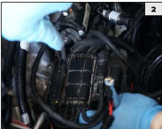
Remove wire loom housing bolts to remove stock low pressure line
