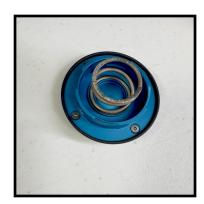
6. Place plastic disc onto spring and press down, keeping the disc mostly flat, until it clicks into place all the way around.
