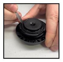
While prying up, slide tool around the body to release the valve. Be aware that there is a spring under tension below, and will shoot the cap off when released. Use your thumb to keep this from happening, but do not press it down.
