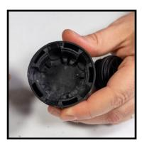
4. Remove screws from top plate on billet cap using a 1.3mm Allen Driver and remove top plate from body.
