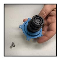
Place cap into main body by lining up the logo with the retaining tab that extends past body as shown in pictures below.
