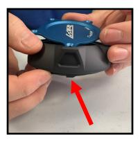
7. Install the 5 M3 screws using a 2mm Allen driver. The first screw should not be tightened at first to allow alignment of a second screw across so that the o-ring does not cause a bind. Tighten all the screws but be careful to not over-tighten or strip the heads, as they are small screws.
