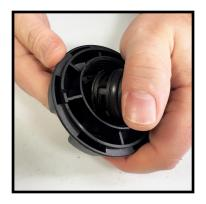
Take apart new billet cap by unscrewing the 5 M3 screws using a 2mm Allen driver.
