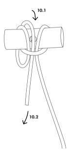
ADJUST THE LENGHT OF THE LEATHER CORD BEFORE MARKING THE HOLE IN THE WOODEN DOWEL. THEN DRILL AND APPLY THE WALL PLUG.
