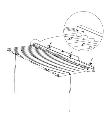
DRILL FOUR HOLES IN THE WALL AT THE MARKED SPOTS
