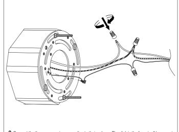
**2.** Connect the three power wires according to their colours. The slick is the live wire (L), coarse is the neutral wire (N), brass is the earth wire  $(\frac{1}{2})$ .
