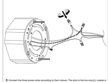
Connect the three power wires according to their colours. The slick is the live wire (L), coarse is the neutral wire (N), brass is the earth wire (±).
