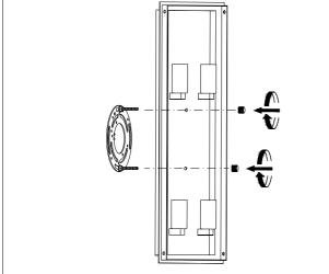
3. Place the wall plate over the crossbar and fix it securely with the screws supplied.
