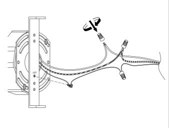
2. Connect the three wires according to their colours. The slick is the live wire (L), coarse the neutral wire (N), brass is the earth wire  $(\frac{1}{-})$ .
