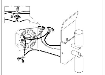
**2.** Connect the 3 wires according to their colours. The slick is the live wire (L), coarse is the neutral wire (N), brass is the earth wire( $\pm$ ).
