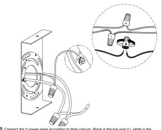
2. Connect the 3 power wires according to their colours. Black is the live wire (L), white is the neutral wire (N) and brass wire is the earth wire (±).
