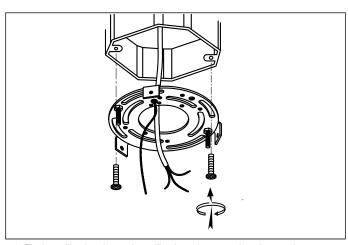
Fix the ceiling bracket to the ceiling by using mounting plugs and screws suitable for your ceiling type.
