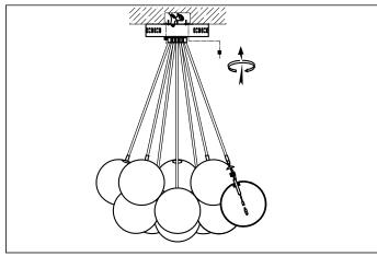
3. Place the lamp over the ceiling plate and fix it with the nuts supplied.
