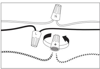
Connect the three wires according to their colours. Black is the live wire, white is the neutral wire, brass is the earth wire.
