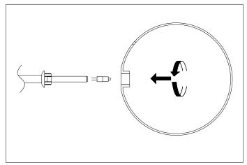
Place the G4 lightbulbs and carefully screw on the glass balls, without overthightening them.
