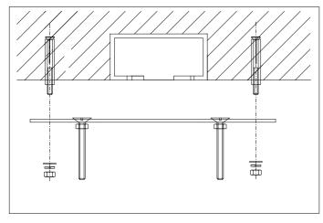
1. Fix the ceiling plate to the ceiling by using bolts and screws suitable to your ceiling type.
