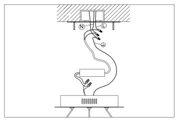
2. Place or hold the lamp in an elevated position in such a way that the wires can freely reach the ceiling junction box. Connect the 3 wires according to their colors. Black is the live wire, white is the neutral wire and brass wire is the earth wire.
