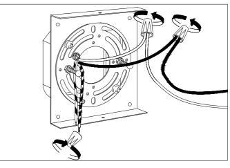
2. Connect the 3 wires according to their colours. Black is the live wire, white is the neutral wire, brass is the earth wire.
