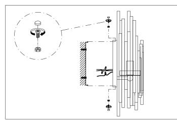
3. Place the lamp over the wall plate and fix it securely with the nuts supplied.
