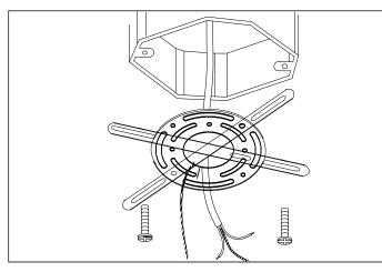
Fix the ceiling plate to the ceiling by using mounting plugs and screws suitable to your ceiling type. Place or hold the lamp in an elevated position in such a way that the wires can freely reach the ceiling junction box.
