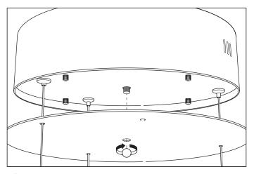
5. Place the ceiling plate over the canopy. Fix the ceiling canopy securely with the nut.
