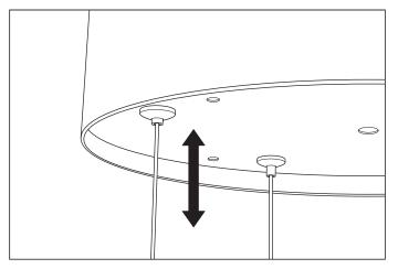
Adjust the height of the steel wires by pressing the wire lock on the ceiling canopy and pulling/pushing the wire through.
