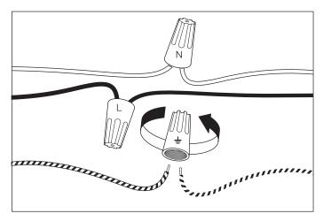
Connect the 3 wires to the LED driver according to their colours. The slick wire is the live wire, the coarse wire is the neutral wire, the brass wire is the earth wire.
