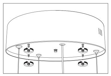
4. Place the ceiling canopy over the crossbar. Fix the ceiling canopy securely with the nuts.
