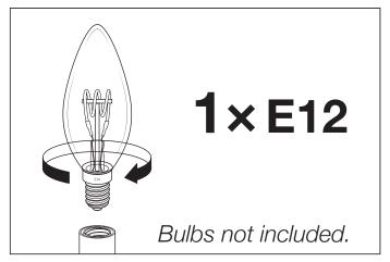
**4.** Carefully place the bulb in the fittings. Do NOT turn the bulb further than necessary, to prevent damage to the fitting.
