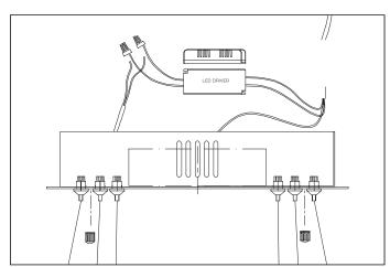
4. Place the canopy over the wall plate and fix it with the four nuts.
