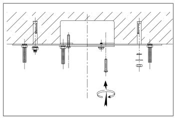
$\textbf{1.} \ \ \text{Fix the bolts to the ceiling. Then fix the ceiling plate to ceiling with screws.}$
