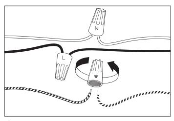
3. Connect the three wires. The slick wire is the live wire, the coarse wire is the neutral wire, brass is the earth wire.
