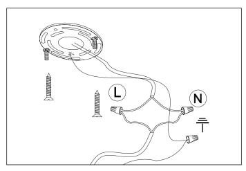
Fix the ceiling plate to the ceiling by using wall mounting plugs and screws suitable for your wall type.
