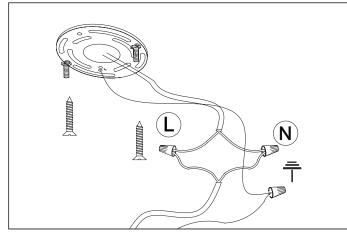
**1.** Fix the ceiling plate to the ceiling by using wall mounting plugs and screws suitable for your wall type.
