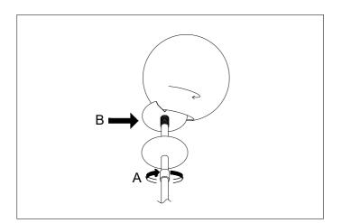
3. Tilt the glass ball so you can place it over one side of part B. Then tilt again so it is completely over part B. Now tighten part A until the glass is secure.
