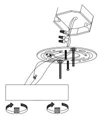
**4** Connect the 3 wires. Connect neutral wire to N, live wire to L and connect the earth wire to the grounding symbol.
