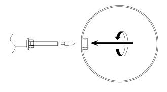
Turn-off the electricity supply at main circuit panel before installing. Do not connect electricity supply until your ceiling light is fully assembled and installed.
