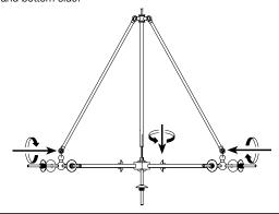
**3** Thread the wire from the lamp through the pipe.
