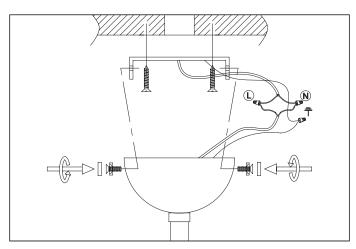
1. Fix the ceiling plate to the ceiling by using mounting plugs and screws suitable to your ceiling type.
