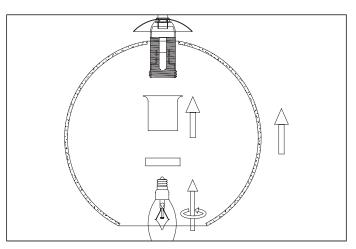
2. Slide the glass over the lampholder. While holding the glass in place slide the metal sleeve over the lampholder and secure it with the ring.
