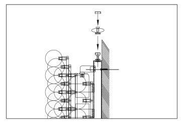
**4.** Place the lamp body over the wall plate and fix it securely with the screws.
