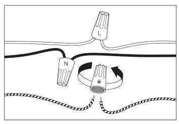
2. Connect the 3 wires according to their colors. Black is the live wire, white is the neutral wire and brass wire is the earth wire.
