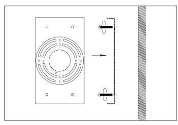
1. Fix the wall plate to the wall by using wall mounting plugs and screws suitable to your wall type.
