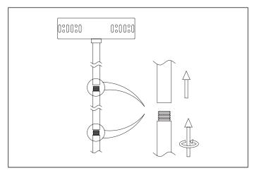
1. Determine the desired height of your chandelier and connect the extension pipes. Thread the wire from the lamp through the pipes. Three pipes are included, extra extension pipes can be ordered.
