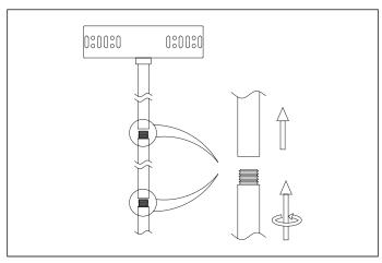
1. Determine the desired height of your chandelier and connect the extension pipes. Thread the wire from the lamp through the pipes. Three pipes are included, extra extension pipes can be ordered.
