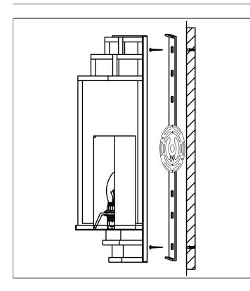
1. Fix the wall plate to the wall by using wall mounting plugs and screws suitable to your wall type.
