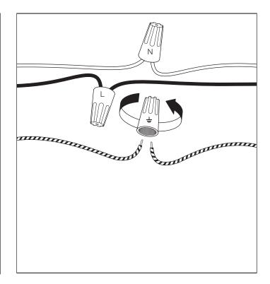
2. Connect the 3 wires according to their colors. Black is the live wire, white is the neutral wire and brass wire is the earth wire.
