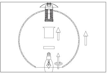
${\bf 2.}$  Slide the glass over the lampholder. While holding the glass in place slide the metal sleeve over the lampholder and secure it with the ring.
