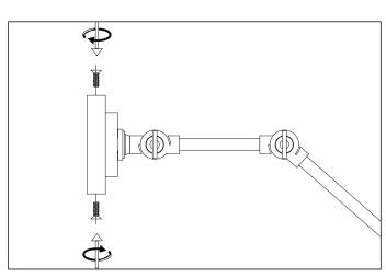
2. Place the lamp over the wall plate and fix it with the screws.
