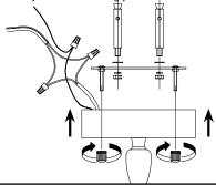
**5** Connect the 3 power wires with the transformer according to their colours. Brown is the live wire, blue is the neutral wire, green/yellow is the earth wire. Place the ceiling canopy flush against the ceiling and fix it securely with the two nuts supplied.
