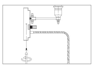
2. Place the lamp over the wall plate and fix it with the screws on the sides.
