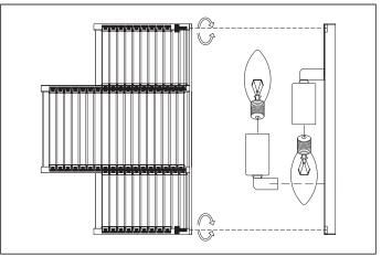
4. Place the lamp over the wall plate and secure with the four nuts.
