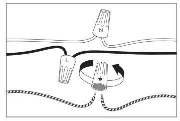
2. Connect the 3 wires according to their colors. Black is the live wire, white is the neutral wire and brass wire is the earth wire.
