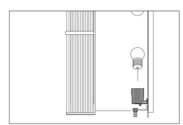
Place the bulbs, than place the lamp over the wall plate and fix it securely with the nuts(B) supplied.
