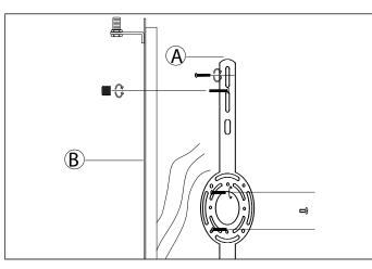
1. Fix the wall plate(A) to the wall by using wall mounting plugs and screws suitable for your wall.
