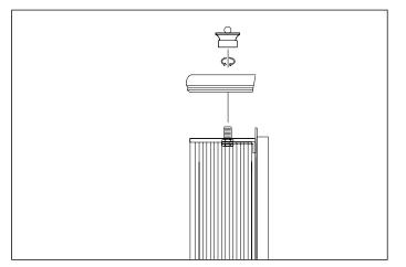
6. Finally place the top cap and secure the it with the finial.
