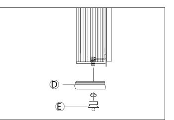
${\bf 5.}$  Place the shade over the lamp and secure it by placing the bottom cap (D) and securing it with the finial (E).
